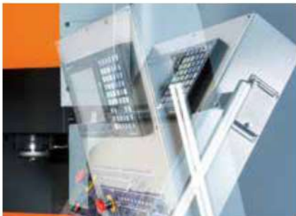
Swivel control panel
